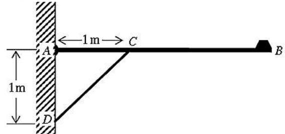
The figure above shows a uniform rod  $AB$ , of length 2.5 m and mass 10 kg, with one of its ends  $A$  smoothly hinged vertical wall. The rod is kept in equilibrium in a horizontal position by a light rigid strut  $DC$ , where  $D$  lies on the same wall vertically below  $A$  and  $C$  lies on the rod such that  $AC = AD = 1 \text{ m}$ . A particle of mass 5 kg is placed at  $B$ . The plane  $ACD$  is perpendicular to the wall.
