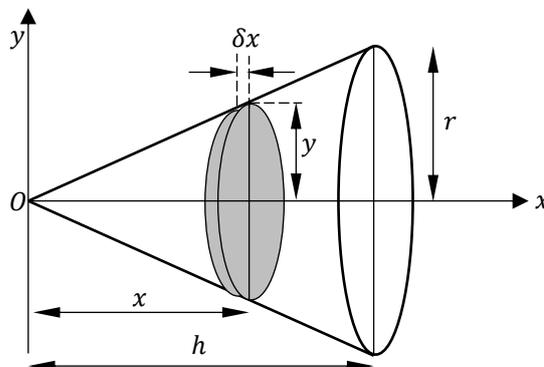
Each cylinder has its centre of mass on the axis  $Ox$ . The radius of each cylinder is  $y$  and the thickness of each cylinder will be  $\delta x$ . So the volume of each cylinder will be  $\pi y^2 \delta x$ .
