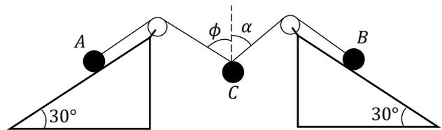
Light inextensible strings attached to A and B pass along the lines of greatest slope, over smooth pulleys and are connected to a third mass C hanging freely. The strings make angles of  $\phi$  and  $\alpha$  with the upward vertical as shown.
