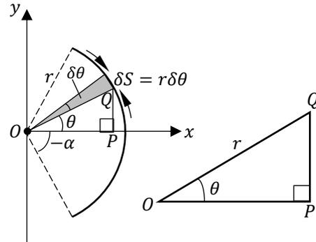
Each small length is  $r \delta \theta$  long. The distance of the centre of mass from  $Oy$  will be  $OP$  since the length  $r \delta \theta$  will be extremely small and so the centre and end of this arc will be negligible distance apart. This is calculated using trigonometry,  $OP = r \cos \theta$ .
