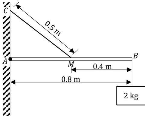
The beam is held in a horizontal position by a light inextensible string of length 0.5 metres. The string joins the mid-point  $M$  of the beam to a point  $C$  vertically above  $A$ . Find the:
