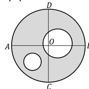
One hole, of radius 20 mm, has its centre on  $OB$  at a distance of 5 mm from  $O$ ; the other, of radius 10 mm, has its centre at a distance of 40 mm from  $OA$  and 20 mm from  $OC$ . Show that the centre of mass of the plate is located on the axis  $COD$  and find its distance from  $O$ .
