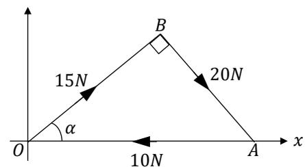
Find the equation of the line of action of the resultant of the forces shown in the diagram, given that  $\tan \alpha = \frac{3}{4}$  and that  $A$  is the point  $(7, 0)$ .
