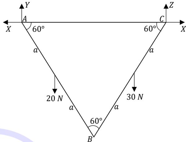
By symmetry, the horizontal reactions at  $A$  and  $C$  must be equal.
