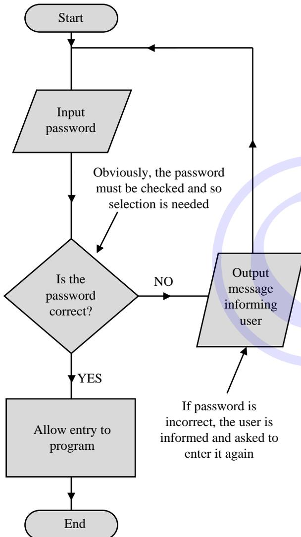
In this flow chart, there is iteration. If the password is incorrect, then in this particular algorithm the user is asked to enter it again, and again, and again, forever or until it is correct.
