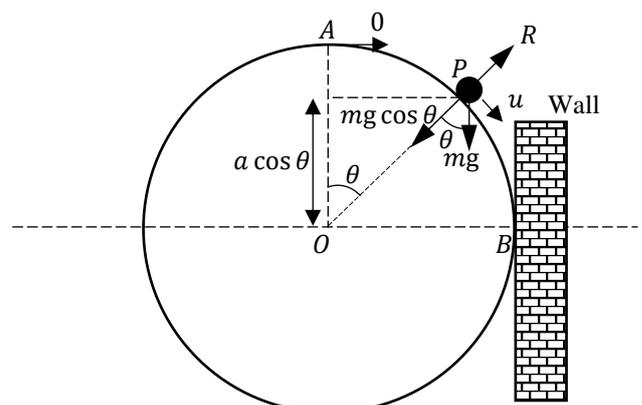
$$(a) \text{ At } B, mg \cos 60^\circ + R = \frac{mv^2}{a}$$
