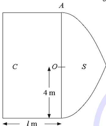
The figure above shows a cross section of a uniform solid  $P$  consisting of two components, a solid cylinder  $C$  and the solid  $S$ . The cylinder  $C$  has radius 4 m and length  $l$  metres. One end of  $C$  coincides with the plane circular face of  $S$ . The point  $A$  is on the circumference of the circular face common to  $C$  and  $S$ . When the solid  $P$  is freely suspended from  $A$ , the solid  $P$  hangs with its axis of symmetry horizontal.
