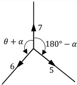
5 N force at  $122.9^\circ$  and 6 N force at  $224.2^\circ$
