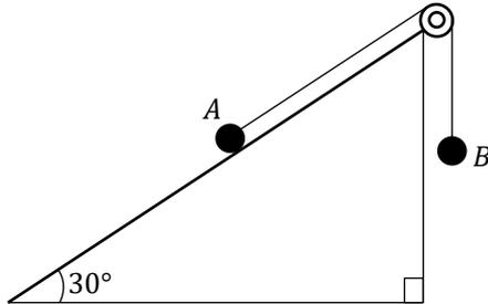
Block  $A$  is resting on a rough plane is inclined at  $30^\circ$  to the horizontal while block  $B$  hangs freely. When the system is released from rest, block  $B$  travels a distance of 0.75 m before it attains a speed of  $2.25 \text{ ms}^{-1}$ . Calculate the
