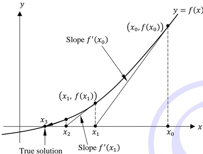
From the geometric picture, we can develop an algebraic formula for Newton's method. The tangent line at  $x_0$  has slope given by the derivative  $f'(x_0)$ . One point on the tangent line is  $(x_0, f(x_0))$ .
