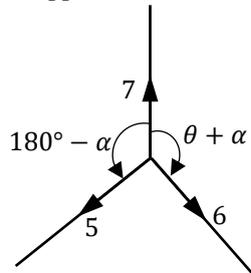
6 N force at  $136^\circ$  and 5 N force at  $237.1^\circ$
