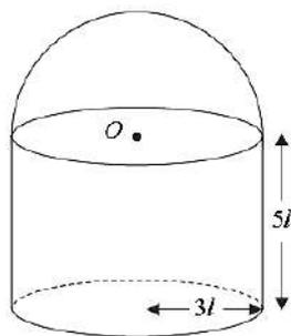
The density of the hemisphere is **twice** the density of the cylinder.
