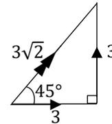
Hence the system is equivalent to a force of  $3\sqrt{2}N$  acting along  $AC$  together with a couple of moment  $6 Nm$  in the sense  $ABCD$ .
