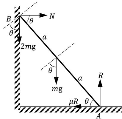
$$\begin{aligned} (\uparrow); R &= 3mg \\ (\rightarrow); N &= \mu R \\ \sim A; mg \cos \theta \times a + 2mg \cos \theta \times 2a &= N \sin \theta \times 2a \\ 5mg \cos \theta &= 2N \sin \theta \\ 5mg \cos \theta &= 2(\mu R) \sin \theta \\ 5mg \cos \theta &= 2 \times \frac{5}{12} \times 3mg \sin \theta \\ \cos \theta &= \frac{1}{2} \sin \theta \\ \tan \theta &= 2 \\ \theta &= 63.4^\circ \end{aligned}$$
