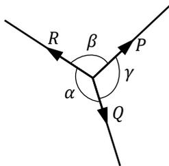
If three concurrent coplanar forces  $P, Q$  and  $R$  are in equilibrium and the angles between  $Q$  and  $R, R$  and  $P, P$  and  $Q$  are  $\alpha, \beta$  and  $\gamma$  respectively as shown, then Lami's theorem states that:
