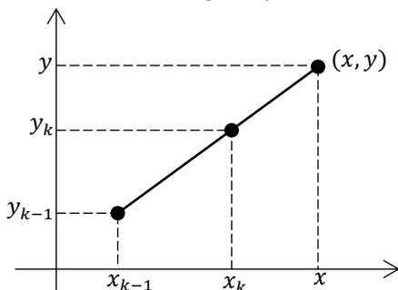
If the two data points nearest the point  $x$ , to be extrapolated are  $(x_{k-1}, y_{k-1})$  and  $(x_k, y_k)$ , equating the slopes gives
