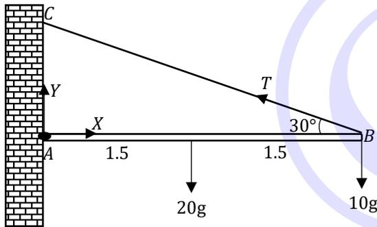
$$\begin{aligned} (\uparrow); Y + T \sin 30^\circ &= 20g + 10g \\ (\rightarrow); X &= T \cos 30^\circ \\ \sim A; (20g \times 1.5) + (10g \times 3) &= T \sin 30^\circ \times 3 \\ 30g + 30g &= \frac{3}{2}T \\ \frac{3}{2}T &= 60g \\ T &= 40g = 392 \text{ N} \end{aligned}$$
