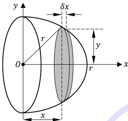
Each cylinder has its centre of mass on the axis  $Ox$ . The radius of each cylinder is  $y$  and the thickness of each cylinder will be  $\delta x$ . So the volume of each cylinder will be  $\pi y^2 \delta x$ .
