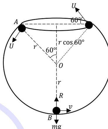
Let the speed of the particle as it passes through  $B$  be  $v$
