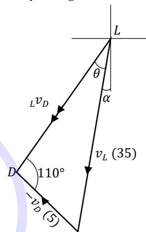
In the velocity triangle;  ${}_L v_D = v_L - v_D$
