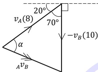
From the velocity triangle,  ${}_A v_B = v_A - v_B$
