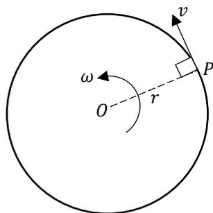
The **linear velocity**  $v$  of  $P$  is directed along the tangent to the circle at  $P$ .
