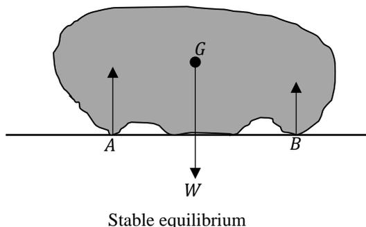
The body will **topple** if the line of action of the weight force lies outside one of these extreme points of contact. It will topple about the point of contact nearest to the line of action of its weight
