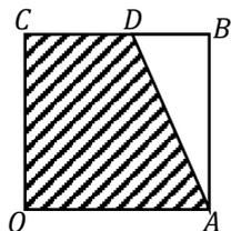
With respect to  $OA$  and  $OC$  as axes, find the coordinates of the centre of mass of a uniform lamina in the form of the figure  $OADC$ .
