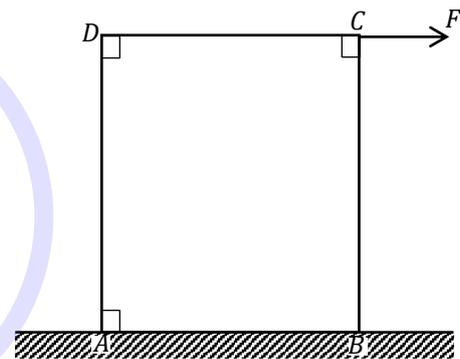
An increasing force,  $F$ , parallel to the table is applied on the upper edge. If the coefficient of friction between the block and the table is 0.7, show that the block will tilt before sliding.
