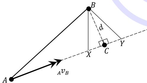
The right-angled triangle  $ABC$  can be used to calculate the shortest distance,  $BC$ . The time to arrive at point  $C$  can be found using
