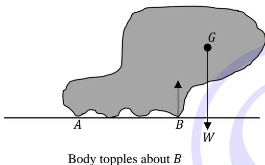
If the body is on a rough inclined plane, it will **topple** if the line of action of the weight force lies outside the lower point of contact of the body with the plane.
