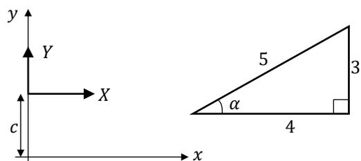
Let  $X$  and  $Y$  be the components of the resultant in the directions of the  $x$ - and  $y$ - axes respectively. Let the line of action cut the  $y$ -axis at the point  $(0, c)$ .
