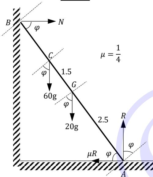
$$\begin{aligned} (\uparrow); R &= 60g + 20g = 80g \\ (\rightarrow); N &= \mu R \\ \sim A; 20g \cos \varphi \times 2.5 + 60g \cos \varphi \times 4 &= N \sin \varphi \times 5 \\ 290g \cos \varphi &= 5(\mu R) \sin \varphi \\ 240g \cos \varphi &= 5\left(\frac{1}{4} \times 80g\right) \sin \varphi \\ \tan \varphi &= 2.9 \\ \varphi &= \tan^{-1} 2.9 = 71^\circ \end{aligned}$$
