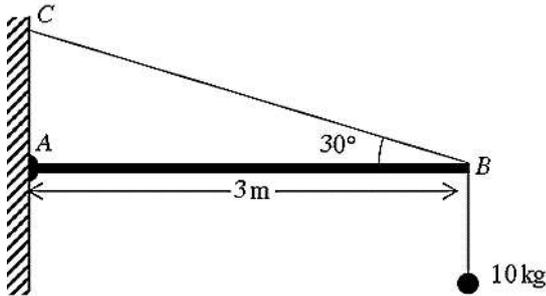
The figure above shows a uniform rod  $AB$ , of length 3 m and of mass 20 kg, smoothly hinged at the point  $A$ , which lies on a vertical wall. A particle, of mass 10 kg, is suspended from the end  $B$  of the rod. The rod is kept in a horizontal position by a light inextensible string  $BC$ , where  $C$  lies on the same wall vertically above  $A$ . The plane  $ABC$  is perpendicular to the wall and the angle  $ABC$  is  $30^\circ$ .
