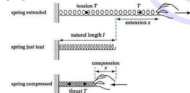
When springs are stretched, they are also subject to Hooke's law. When springs are **compressed**, they exert a **thrust** outward. Hooke's law still applies, but now  $T$  represents the thrust and  $x$  is the compression.
