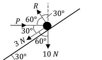
A particle on a slope is subject to the forces shown in the diagram above and is in equilibrium. Find the forces  $R$  and  $P$ .
