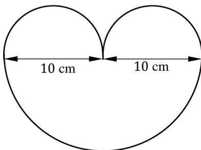
Find the centre of gravity of the lamina made of three semicircles as shown above.
