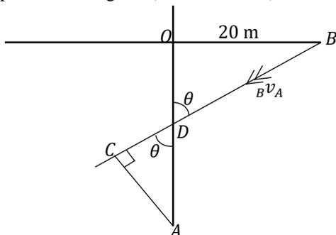
$A$  sees  $B$  travelling along the direction  $BC$ . The cyclists are closest together when  $A$  sees  $B$  to be at a position  $C$ , where  $AC$  is perpendicular to  $BC$ . The shortest distance apart is therefore  $AC$
