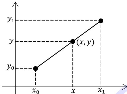
For a value  $x$  in the interval  $(x_0, x_1)$ , the value  $y$  along the straight line is given by from the equation of slopes which can be derived geometrically from the figure above
