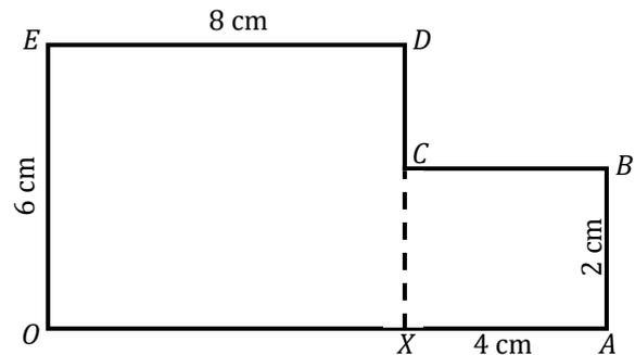
Find the centre of mass of the above uniform lamina taking  $OA$  and  $OE$  as axes
