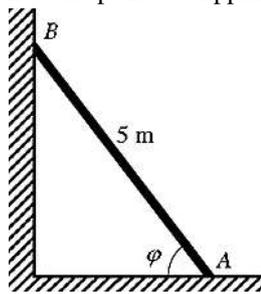
Given that the coefficient of friction between the ladder and the ground is  $\frac{1}{4}$ , find the value of  $\varphi$ , to the nearest degree.
