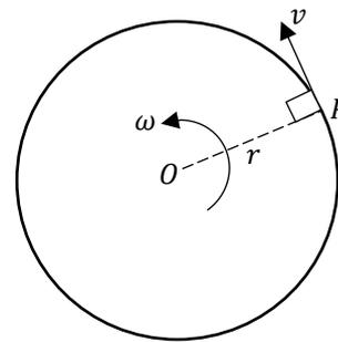
When a particle  $P$ , of mass  $m$  is moving in a vertical circle, centre  $O$ , radius  $r$ , its speed  $v$  is variable.
