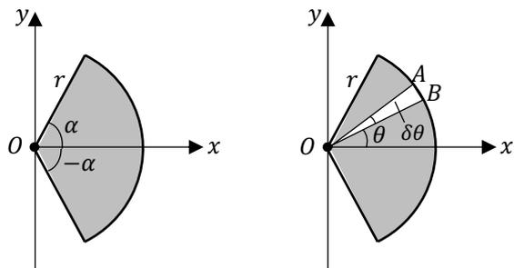
Element  $OAB$  subtends an angle  $\delta\theta$  (in radians) at  $O$ . By considering this element as a triangle and by allowing  $\theta$  to range from  $-\alpha$  to  $+\alpha$ , the centre of mass can be obtained as follows.
