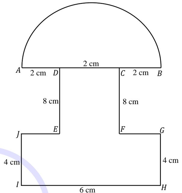
The figure  $ABCDEFGHIJ$  shows a symmetrical composite lamina made up of a semi-circle, radius 3 cm, a rectangle  $CDEF$   $2 \text{ cm} \times 8 \text{ cm}$  and another rectangle  $GHIJ$   $6 \text{ cm} \times 4 \text{ cm}$ .
