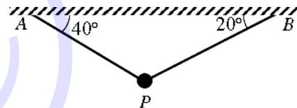
A particle  $P$  of weight  $60\text{ N}$  is suspended by two strings from a fixed horizontal ceiling. The particle hangs in equilibrium. The strings are light and inextensible and are inclined at  $40^\circ$  and  $20^\circ$  to the ceiling, as shown in the figure above. Find the tension in each of the two strings.
