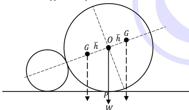
It is clear that for the toy to return to its vertical position, the point of action of its weight must lie on the left of  $P$  i.e.  $\bar{h} < 0$
