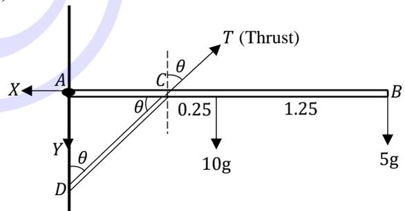
$$\begin{aligned} ACD \text{ is right angled and isosceles, } \therefore \theta &= 45^\circ \\ (\uparrow); T \sin \theta &= Y + 10g + 5g \\ (\rightarrow); X &= T \cos \theta \\ \sim A; T \sin \theta \times 1 &= 10g \times 1.25 + 5g \times 2.5 \end{aligned}$$
