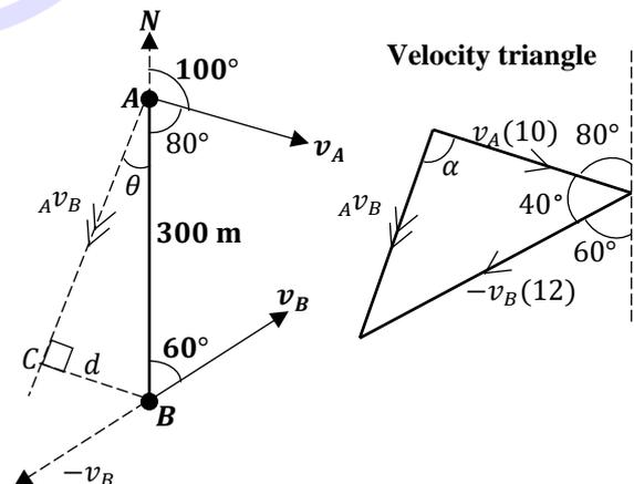
From the velocity triangle;  $_A v_B = v_A - v_B$
