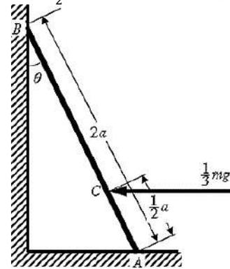
The angle between the ladder and the vertical wall is  $\theta$ . By modelling the ladder as a uniform rod show that  $\tan \theta = \frac{1}{2}$ .
