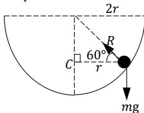
$$\begin{aligned} \uparrow R \sin 60^\circ &= mg \\ \leftarrow R \cos 60^\circ &= m\omega^2 r \\ \tan 60^\circ &= \frac{g}{\omega^2 r} \\ \omega^2 &= \frac{g}{r \tan 60^\circ} = \frac{g}{r(\sqrt{3})} \\ \omega &= \sqrt{\frac{g}{r(\sqrt{3})}} = \sqrt{\frac{g\sqrt{3}}{3r}} \end{aligned}$$
