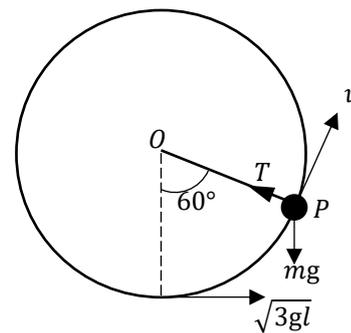
Height of  $P$  when the string is inclined at  $60^\circ$  is given by  $h = l - l \cos 60^\circ = l(1 - \cos 60^\circ)$
