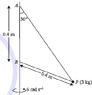
A particle  $P$  of mass 3 kg is attached by two light inextensible strings to two fixed points  $A$  and  $B$  on a fixed vertical pole. Both strings are taut and  $P$  is moving in a horizontal circle with constant angular speed  $6 \text{ rad s}^{-1}$ . String  $AP$  is inclined at  $30^\circ$  to the vertical. String  $BP$  has length 0.4 m and  $A$  is 0.4 m vertically above  $B$ , as shown above. Find the tension in
