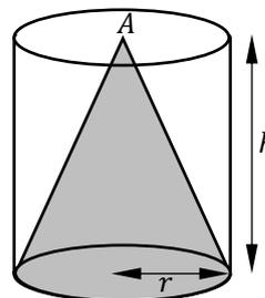
Show that the centre of gravity of the resulting solid is at a distance of  $\frac{3h}{8}$  from the point  $A$  measured along the axis of symmetry.
