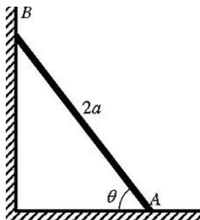
The figure above shows a uniform ladder  $AB$  of length  $2a$  and of mass  $m$  resting with the end  $A$  on rough horizontal ground and the end  $B$  against a smooth vertical wall. The ladder is inclined at an angle  $\theta$  to the ground. When a child of mass  $2m$  is standing on the ladder at  $B$ , the ladder is about
