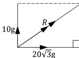
$$\begin{aligned} \text{Total reaction, } R &= \sqrt{(10g)^2 + (20\sqrt{3}g)^2} \\ &= \sqrt{100g^2 + 1200g^2} \\ &= \sqrt{1300g^2} \\ &= \sqrt{100g^2} \times \sqrt{13} \\ &= 10g\sqrt{13} \\ &= 98\sqrt{13} \text{ N} \end{aligned}$$
