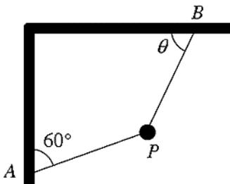
A particle  $P$ , of weight  $300\text{ N}$ , is hanging in equilibrium by two light inextensible strings,  $AP$  and  $BP$ , which lie in the same vertical plane. It is further given that  $AP$  forms an angle of  $60^\circ$  with a vertical wall and  $BP$  forms an angle  $\theta$  with a horizontal ceiling. Calculate the value of  $\theta$  and the tension in  $BP$ , if the tension in  $AP$  is  $120\text{ N}$ .
