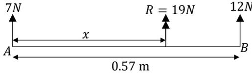
In the given diagram, find the distance  $x$  of the resultant  $R$  from the point  $A$ .
