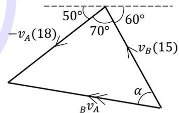
From the velocity triangle;  ${}_B v_A = v_B - v_A$
