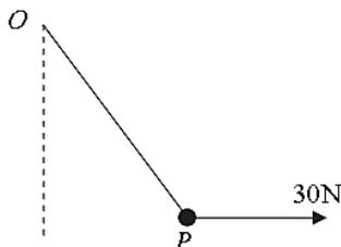
Given that the particle  $P$  is in equilibrium and the elastic energy stored in the string is 10 J, calculate the length  $OP$
