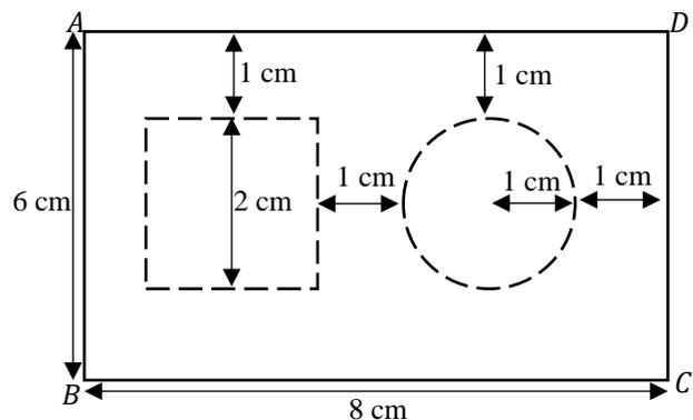
$ABCD$  is uniform rectangular sheet of cardboard of length 8 cm and width 6 cm. A square and a circular hole are cut off from the cardboard as shown above. Calculate the position of the centre of gravity of the remaining sheet. [1999, No. 16: Ans: 3.944 cm from  $AB$  2.825 cm from  $BC$ ]
