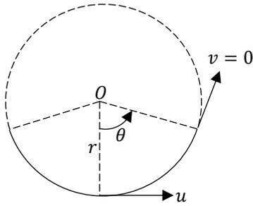
2. The particle **can leave the circular path** and become a projectile e.g. a particle attached to a string, a body moving on the inside/outside surface of a sphere, etc. The particle can do one of these three things. ( $T$  is the tension in the string or normal reaction)
